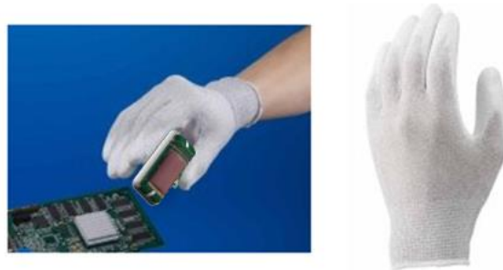
Figure 9. ESD protection glove and handling guide
