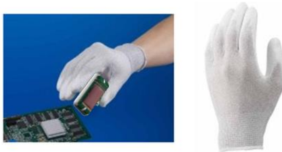
Figure 9. ESD protection glove and handling guide
